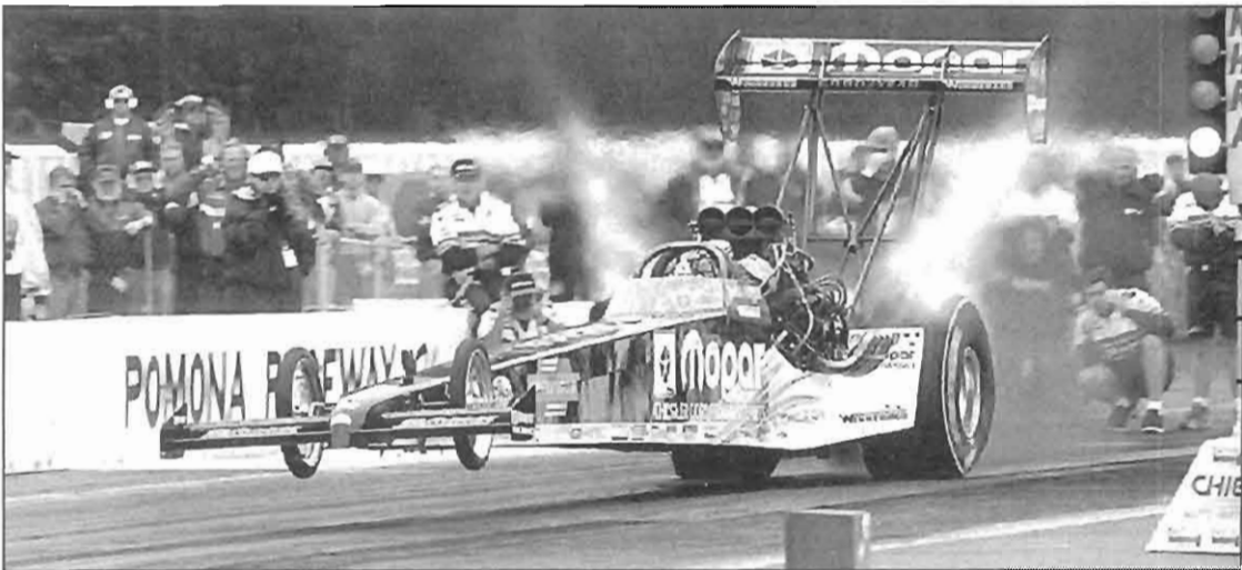
(Above) Darrell Gwynn's Mopar-backed Top Fueler is involved in blower-belt testing for Gates Rubber Co. Other cars involved are the Top Fuel dragsters of Eddie Hill, Kenny Bernstein, and Cory McClenathan and Cruz Pedregon's Funny Car. (Left) The service life of today's supercharger drive belt is normally about four runs at most tracks. Gates has collected hundreds of used belts from Top Fuel and Funny Car teams for testing at the Gates Belt Testing Laboratory in Denver. This year, the company will test about 200 broken belts for tensile strength.
