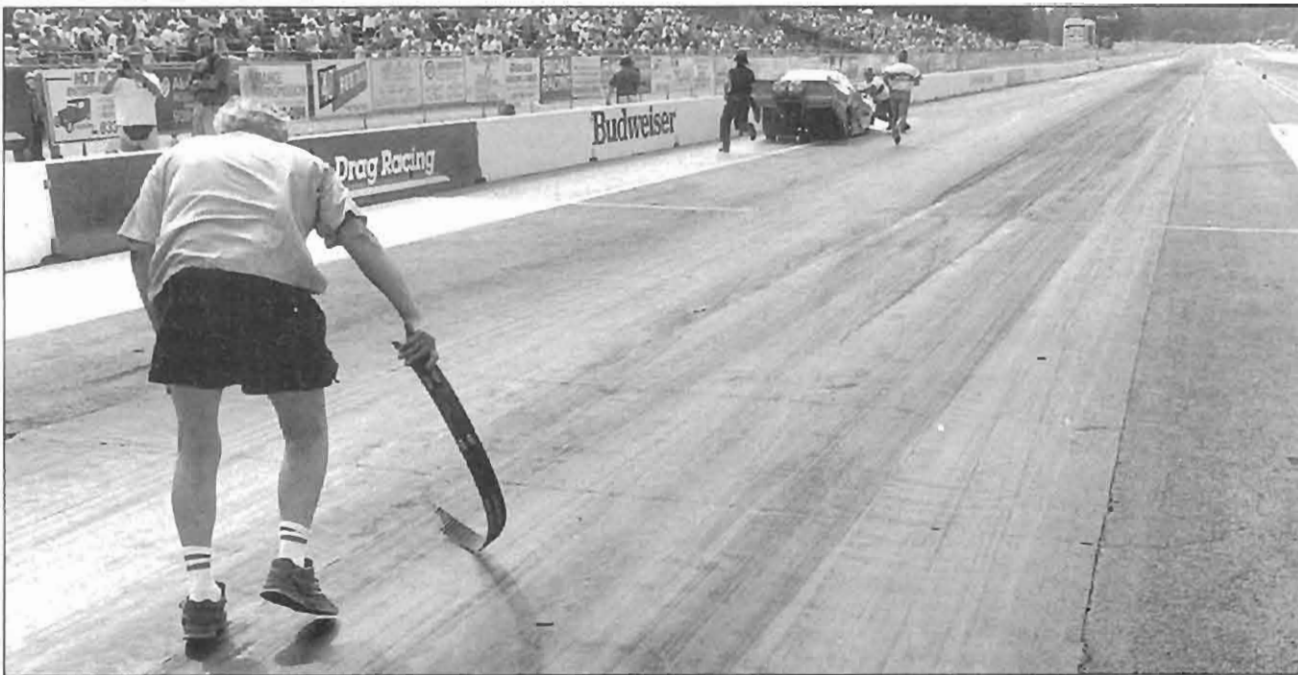
(Above) Darrell Gwynn's Mopar-backed Top Fueler is involved in blower-belt testing for Gates Rubber Co. Other cars involved are the Top Fuel dragsters of Eddie Hill, Kenny Bernstein, and Cory McClenathan and Cruz Pedregon's Funny Car. (Left) The service life of today's supercharger drive belt is normally about four runs at most tracks. Gates has collected hundreds of used belts from Top Fuel and Funny Car teams for testing at the Gates Belt Testing Laboratory in Denver. This year, the company will test about 200 broken belts for tensile strength.
